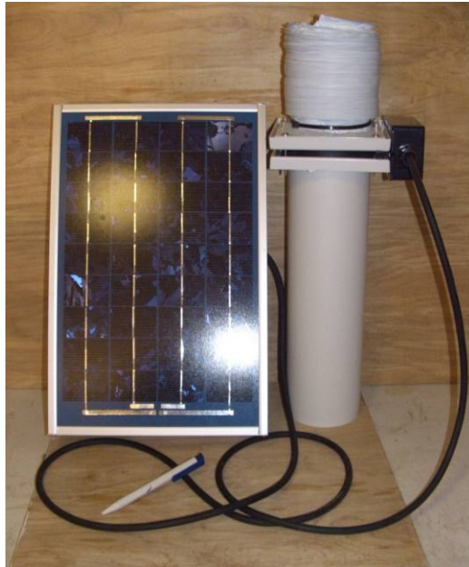
Fan and module assembly (note pen in foreground for scale)
